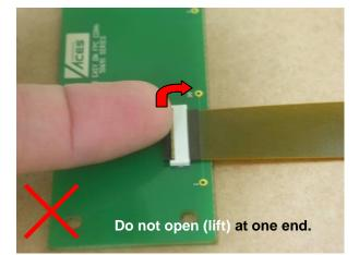
• The actuator opens by rotating it in the direction OPPOSITE to the direction of the insertion of the FPC. DO NOT attempt to open it from the same side as the insertion of the FPC.
