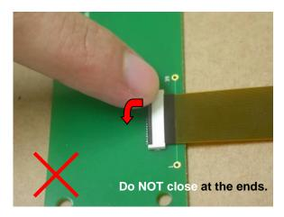
About the lock operation When you lock, it is recommended what the actuator does as a whole, and the actuator was shut surely.
